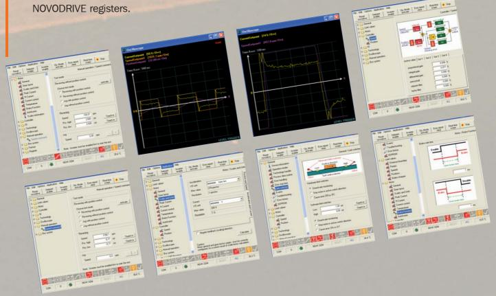
By means of the integrated 4-channel-oscilloscope, all control parameters such as acceleration ramps, limit values, or values for input/output current can be recorded, printed and archived.
